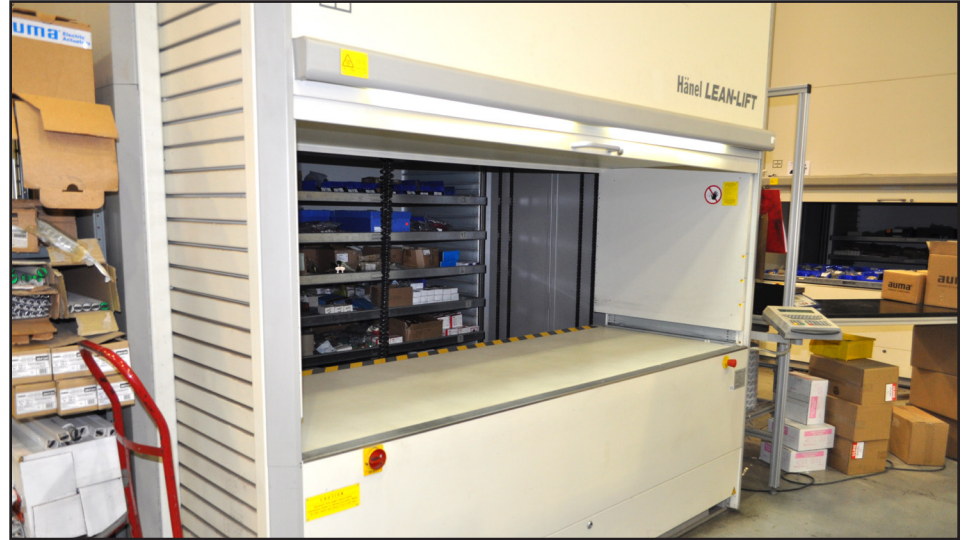
Thousands of parts for assembly operations are stored in this Lean-Lift VLM.
